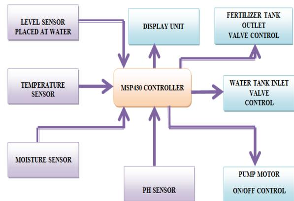
Arduino microcontroller performs corrective actions according to the results of sensors and intimates the relay. The relay triggers the motor with the indication of fertilizer supply duration. Fertilizer is supplied appropriately to the plant by analyzing the recorded values from pH table. Nutrient content of the soil is maintained based on the standard requirement of the plant. The continuous monitoring of nutrient supply can be viewed in web page created through IOT.
