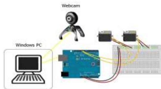
The authenticated image is used to turn ON . If the wrong image is detected, the bike will not start. To turn on for emergency purpose by any other person (known by the authenticated person) the unlock system is provide with the use of keypad numbering system.
