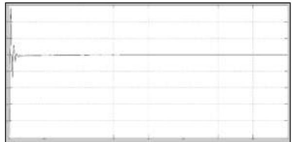
Figure-18: Step response of the system with PID controller tuned using Ziegler Nichols Method
