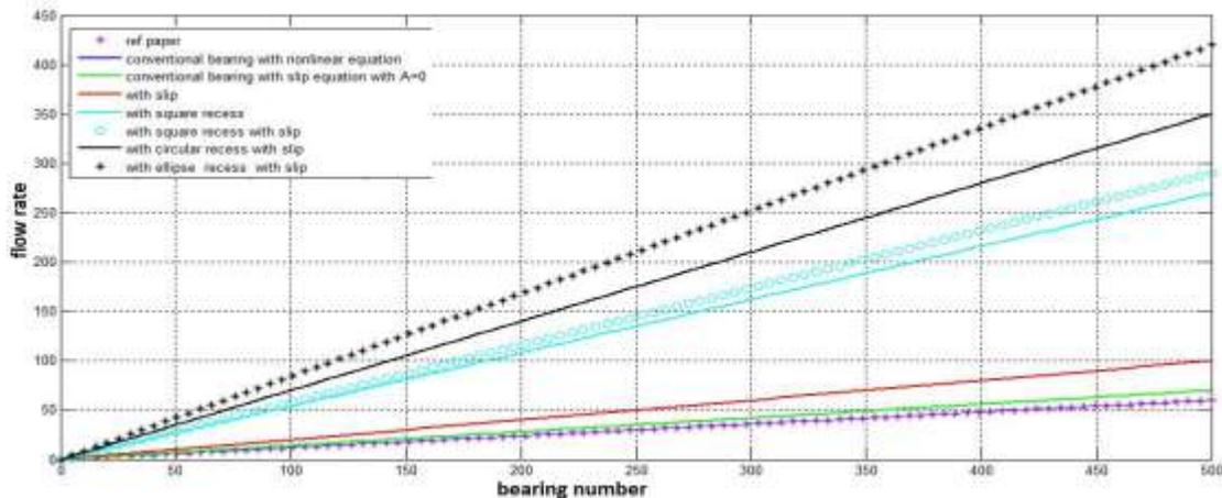
Chart -5: Correlate of flow rate for different values of bearing number for all patterns in slider.
