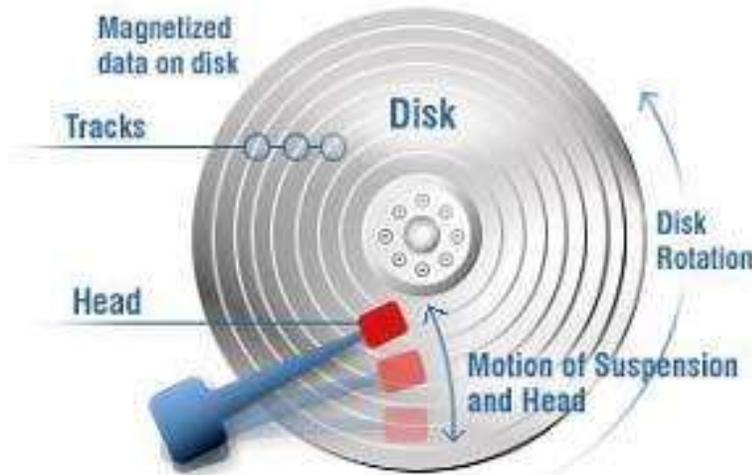
Fig -1: Disc drive using slider [2]
