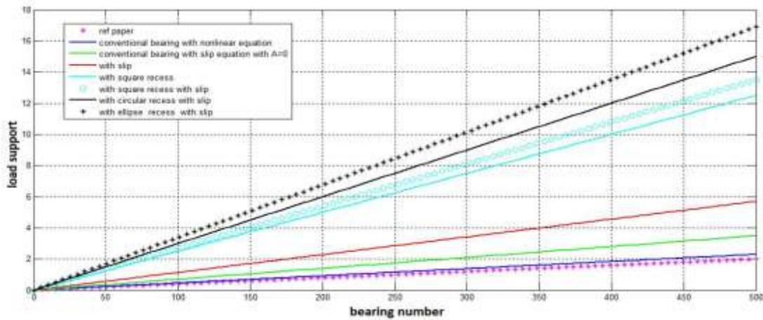
Chart -4: Correlate Load support for different values of bearing number for all patterns in slider.
