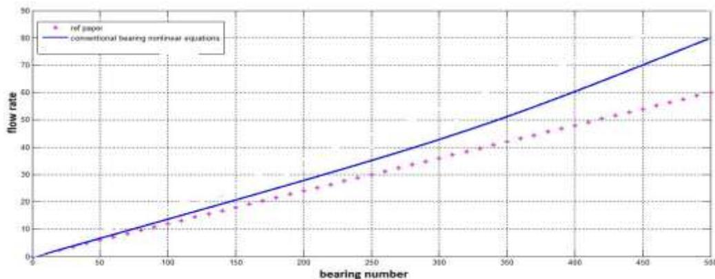
Chart -2: Flow rate of air with respect to bearing number
