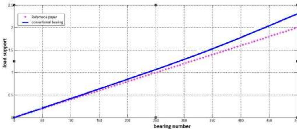
Chart -1: Load support vs. bearing number for simple slider.
