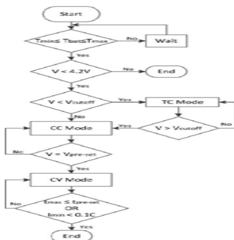
Fig-6: Flow chart of CC/CV charger for Li-ion batteries, where 4.2V corresponds to the maximum cell voltage [17]
