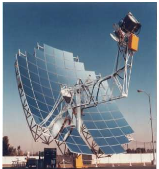
Fig 5 – Stirling engines for low-temperature solar-thermal-electric power generation
