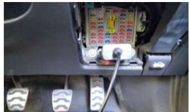
Fig -4: OBD scanner connected to OBD port in the car
