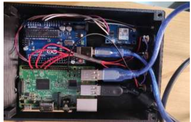
Fig -3: Raspberry-Pi board connected to Arduino Rev 3 Board and enclosed in fiber material
