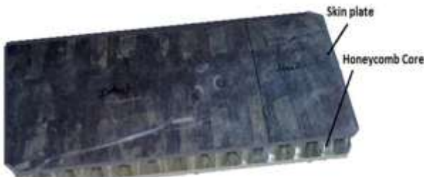
Fig-12: Specimen of Honeycomb Structure
