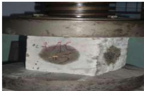
Fig -3: Compressive Strength Testing Arrangement
