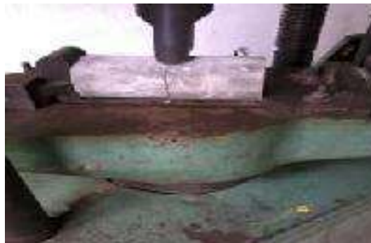
Fig -4: Split Tensile Strength Testing Arrangement
