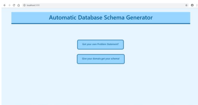
Figure -3: Automatic Database Schema Generator can generate schema from customised problem statement provided by user or from the domain type of user requirement. (For e.g.: User may give a problem statement for Library system as input or only specify 'Library' as domain)
