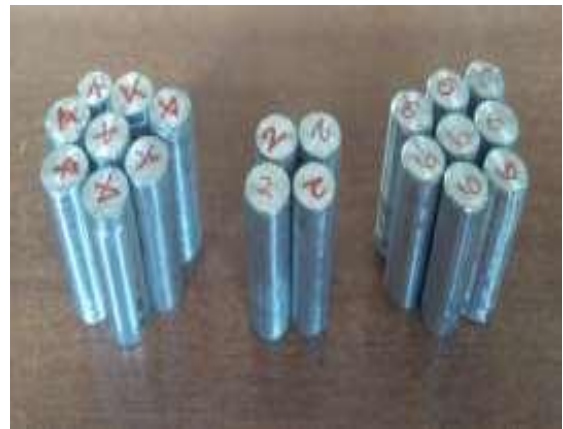
Fig 2.Specimen Pin For Wear Test.
