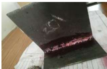
Fig -9: Application of Penetrant
