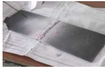
Fig -10: Excess Penetrant Removal
