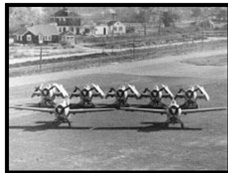
Fig4:-Comparison of the Grumman F4F Wildcat between folded and unfolded wings.
