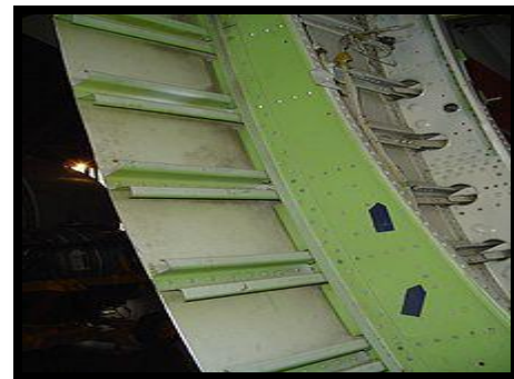
Fig2 :-Sectioned fuselage showing frames, stringers and skin all made of aluminum
