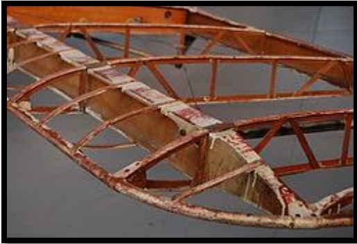
Fig5:-Wing ribs of a de Havilland DH.60 Moth
