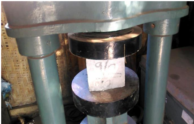
Figure no. 2 Testing of Cube at Site
