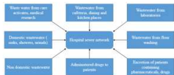
Fig -1: Flowchart of sources of wastewater generation in hospital
