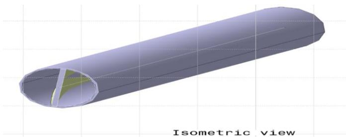
Fig 1. Views of Twisted Tube Insert
