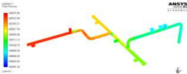
Fig-13: Pathline covered by pressure in Booster pump pipeline for Case I
