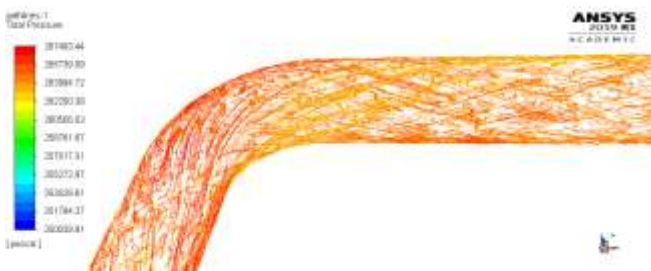
Fig-30: Pathline covered by velocity in Strainer and sample point pipeline for Case III
