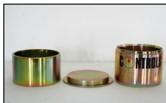
Fig.7 &8: Marshall Stability Specimen moulds
