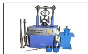
Fig.7 &8: Marshall Stability Specimen moulds
