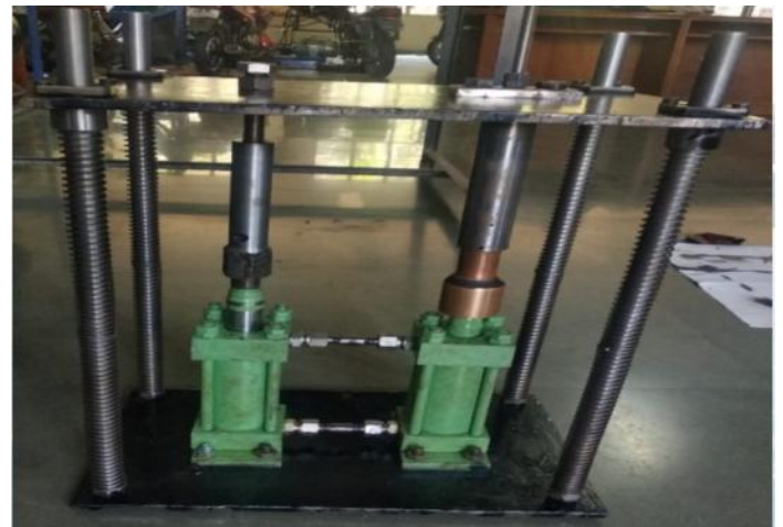
Fig -15: Eddy current damper setup
