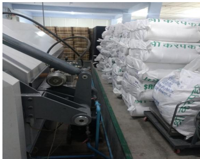
Figure 3.2 Stacking material near moving machinery
