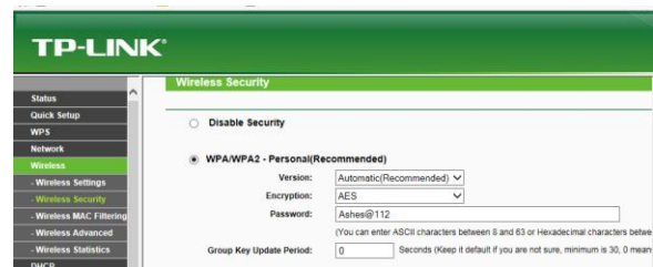
Figure 13: The AP configured to support WPA/ WPA-2 PSK with password "Ashes@112"
