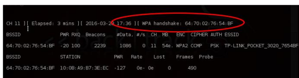
Figure 17: The capturing of the four-way EAPOL handshake as soon as a legitimate client connects to the legitimate AP
