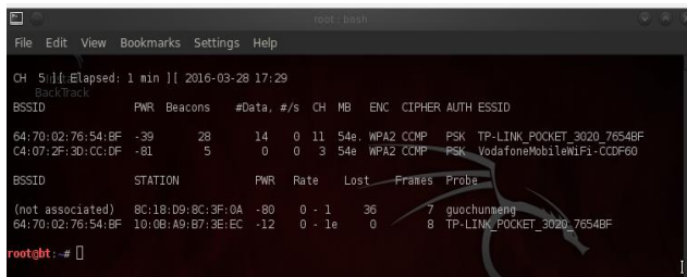
Figure 15: The output of “airodump-ng” used to monitor broadcasting SSIDs
