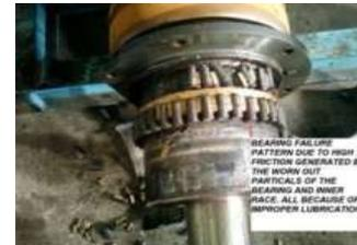
**Fig-12** Bearing Failure Caused Due To Excessive Friction between Bearing and Inner Race.
