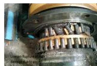
**Fig-13** Uneven Rupture of cage damage due to poor lubrication
