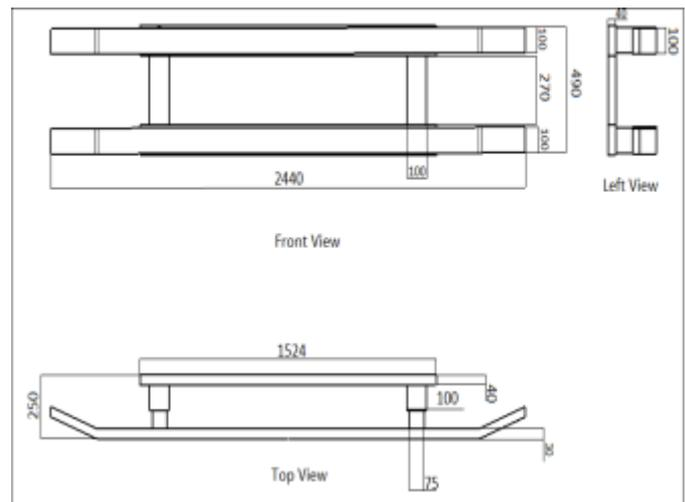
Figure 5: Proposed Design of High Energy Safety Impact Guard
