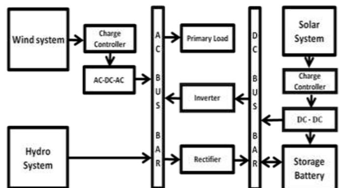
Figure1. Structure of hybrid wind-PV-hydro power generation system
