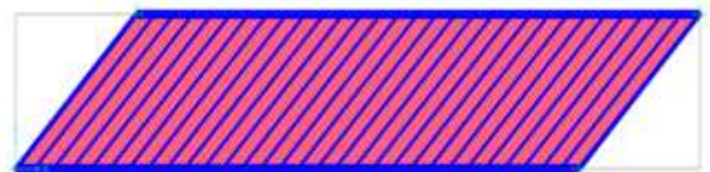
Fig-5: Bottom Plan of the Bridge for 45 degree skew angle
