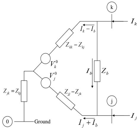
Figure 4: Thevenin equivalent circuit by adding a line between two existing buses
