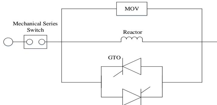
Figure 3: Fault Current Limiter
