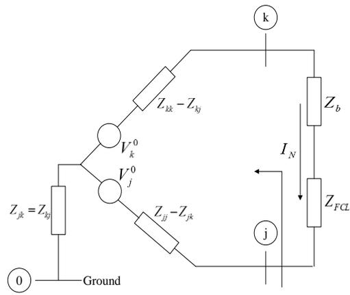
Figure 5: Thevenin equivalent circuit with FCL fired up
