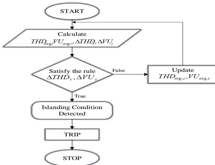
**Figure 2:** Flow Chart for Islanding Detection
