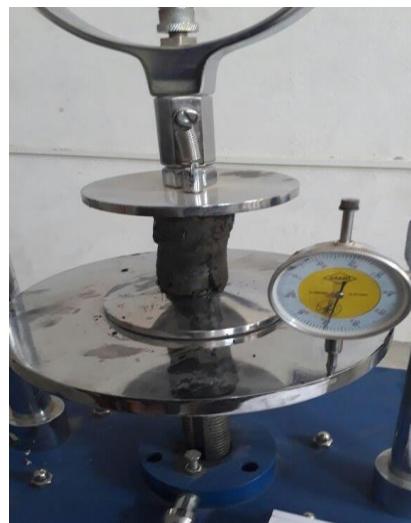
Fig-6 Samples under Loading in UCS apparatus
