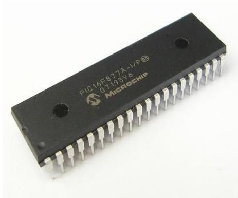
Fig. 2.2: PIC16F877A Microcontroller
