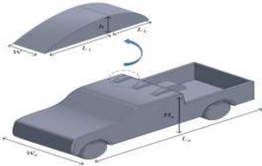
Fig -1: Generic truck test model
