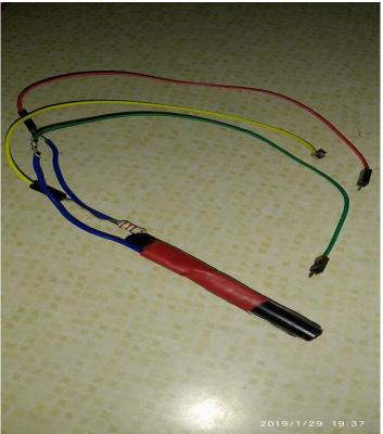
the constant volts. The electrical conductivity is measured by the concentration of dissolved ions which are proportional to the current flow. The dissolved salts concentration is directly proportional to electrical conductivity. The amount of minerals and salts that reside within the water is resulted by the total dissolved solid (TDS). By multiplying the conductivity by a factor of 0.67 B the TDS of water can be determined.
