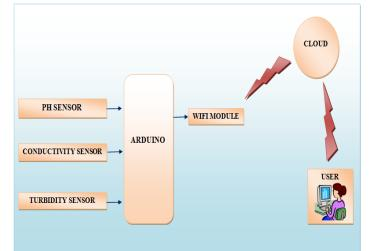
of water goodness by using IoT has been proposed. Internet of things together with the Sensor water meters for the effectiveness, govern the quality of water. Here we are executing, system for monitoring the water goodness through different sensors-turbidity, pH, temperature, conductivity. The controller accesses the information which is monitored by the use of sensors. The accessed data is controlled by the usage of Arduino controller. By using an IoT, the information
