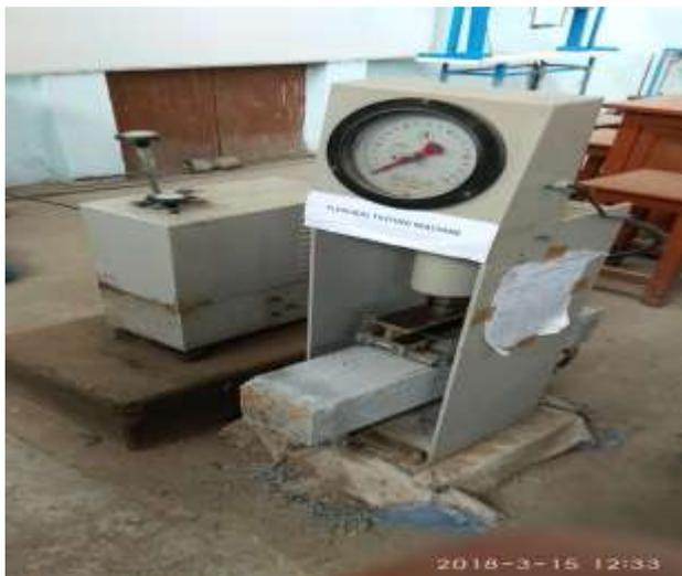
Fig 5: Flexural Strength Test
