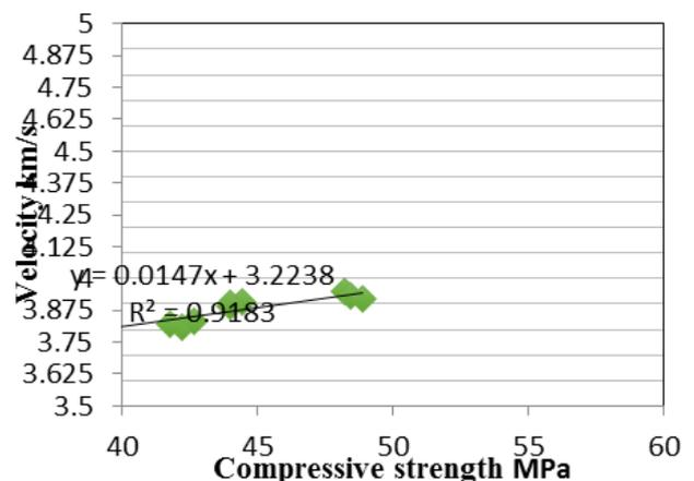
Fig 10: UPV vs Compressive Strength Graph
