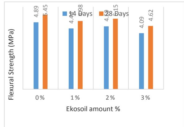
Fig 9: Results of Flexural Strength Test on EKO-PQC Mixes
