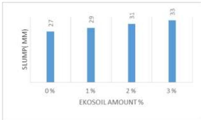
Fig 7: Results of Slump Test on EKO-PQC Mixes
