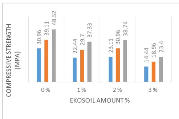
Fig 8: Results of Compressive Strength Test on EKO-PQC mixes
