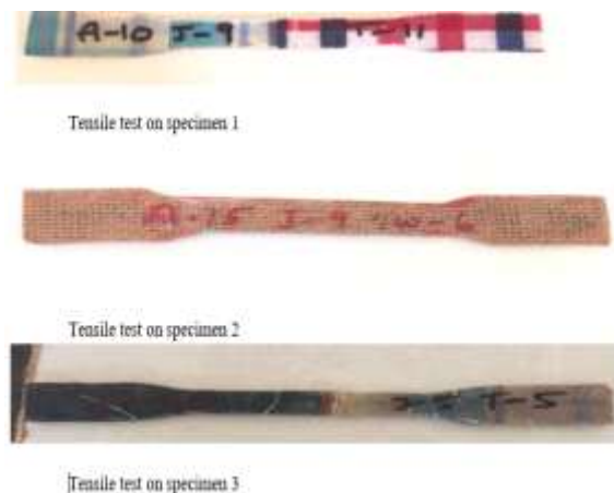
Fig. 2. Shows Dog bone shape Specimens for tensile
