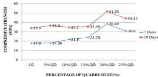
**Chart -1:** compressive strength for various concrete mixes at 7 & 28 days
