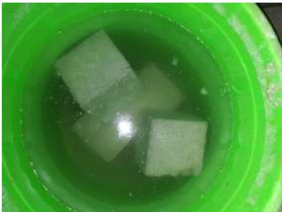
Fig -1: Acid Test on concrete
