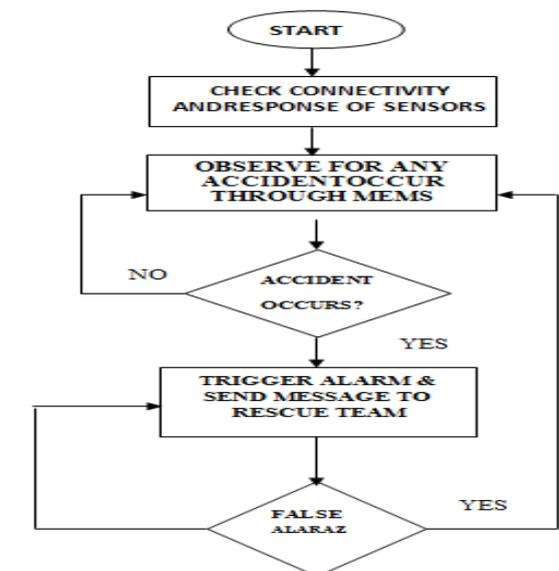
Fig -2 Flow Diagram of Accident Detection system
