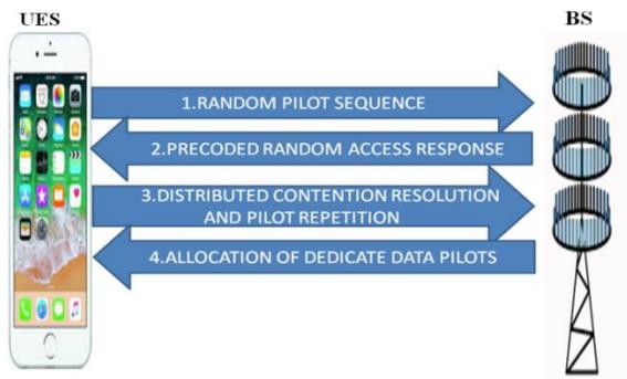
**Fig-9: THE SUCRE RANDOM ACCESS PROTOCOL FOR MASSIVE MIMO.**
