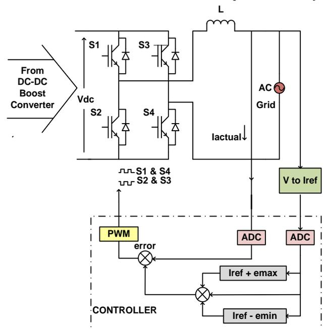
Fig - 6: Hysteresis current control for grid connected inverter
