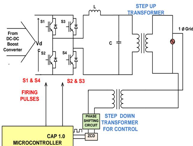
Fig -5: Grid connected inverter using ZCD circuit
