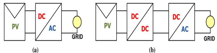
Fig -1: (a) Single stage inverter (b) Multistage inverter
