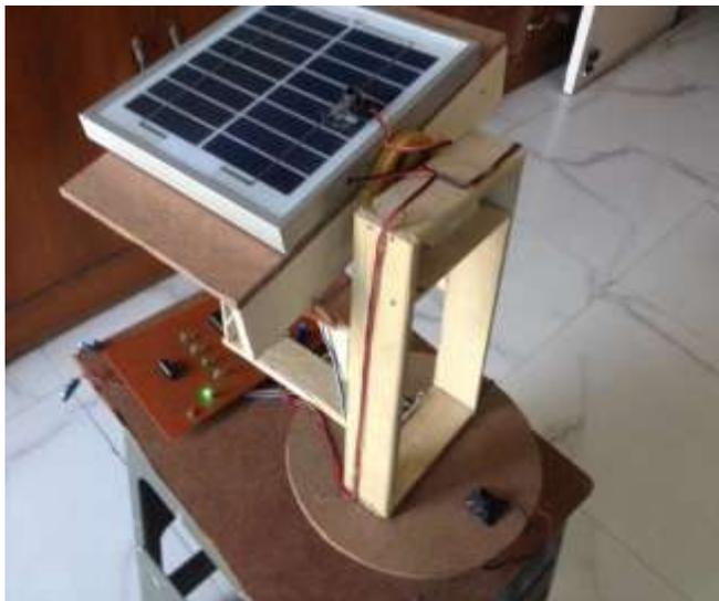
Fig. 3.1.4: Complete Hardware Module of Sun Tracking Solar Panel
