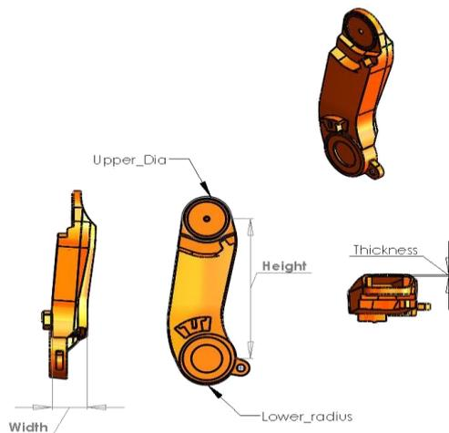
**Fig- 3- Drawing with global parameters**
