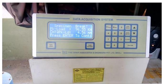
Fig 5: Data Acquisition on UTM for Beam
