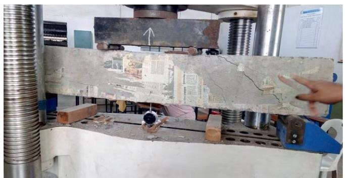
Fig 4: Shear failure and cracks
