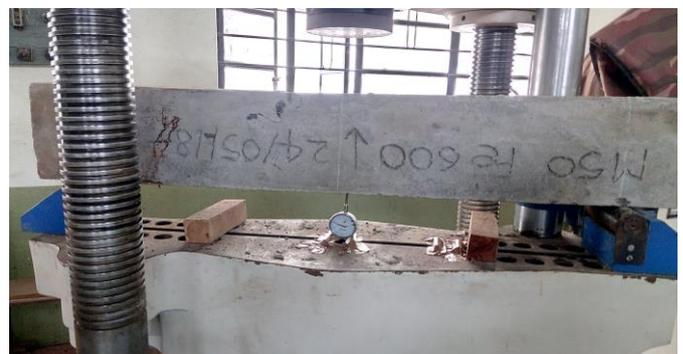
Fig 3: Applying load on Beam
