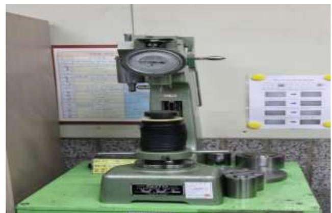
The Brinell method applies a predetermined test load (F) to a carbide ball of fixed diameter (D) which is held for a predetermined time period and then removed. The resulting impression is measured with a specially designed Brinell microscope or optical
