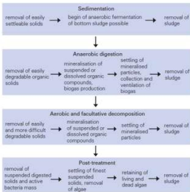
Figure 8: Process of treatment of waste by DEWATS method
