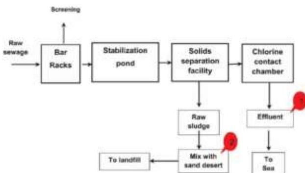
Figure 3: Process of treatment in waste stabilization ponds
