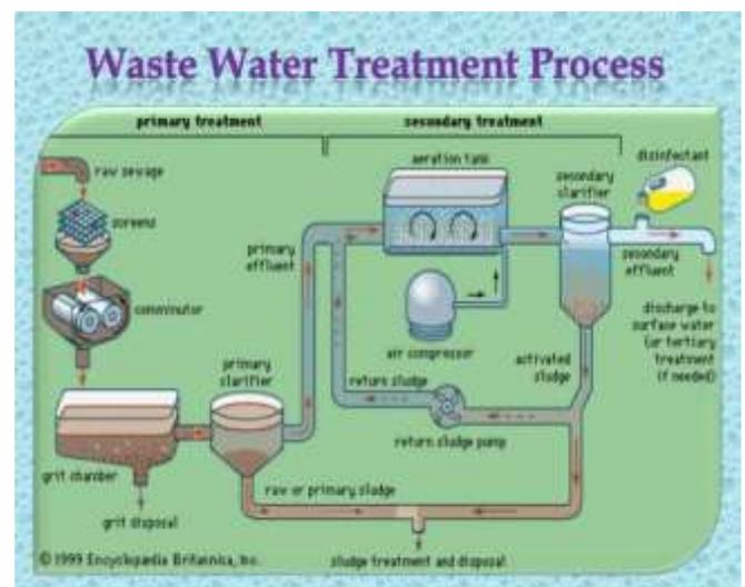
**Figure 2:** waste water Treatment Process
