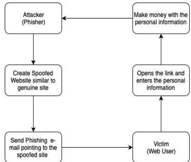
Fig. 1: Flow diagram of phishing attack using e-mail
