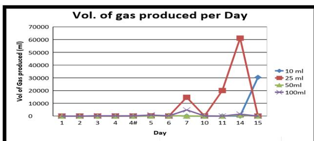
**Fig -5: Daily biogas production of various digesters with various pH # after addition of aliquots of NaOH as per Table No.3**
