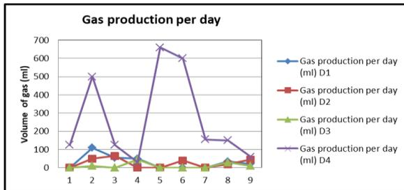
**Fig- 4: Comparison of Daily Biogas production with various additives**
