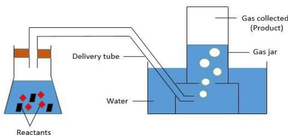
**Fig-1: Schematic diagram of the lab-scale experimental set-up**
