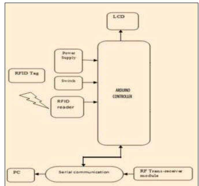
Fig. 5. Block Diagram for Smart Trolley
