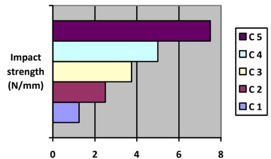
For Izod test conducted on the Palm tree fiber Reinforced with glass fiber were found to be 7.5 N/mm
