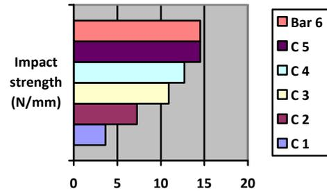
For Charpy test conducted on the Palm tree fiber Reinforced with glass fiber were found to be 14.54 N/mm.
