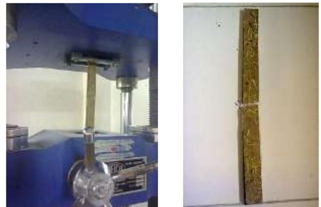
Fig 3.1 tensile test specimen
