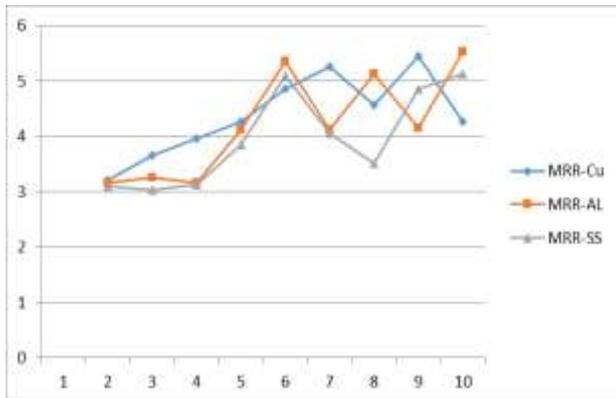
**Comparison of Experimental ELECTRODE WEAR RATE between Copper, Aluminium and SS**
