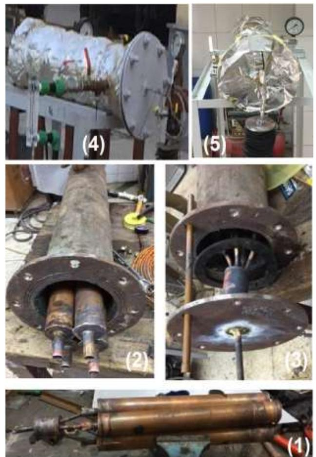
Fig. 2(b) A photographic view of the manufactured adsorbing bed and its assembling
