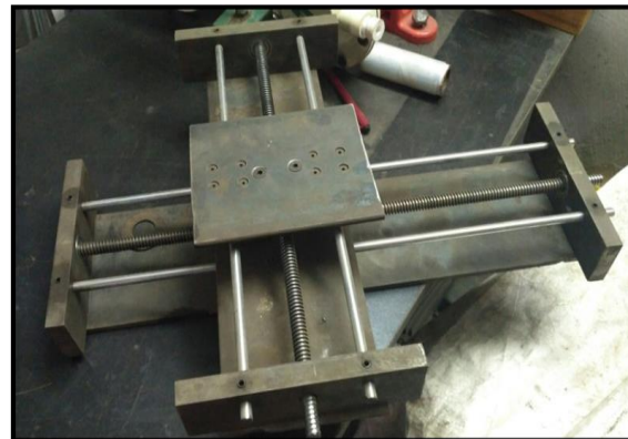
Figure 6: X-Y work table Lead screw Assembly
