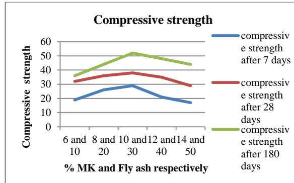
Fig. 1.4 Compressive strength of modified concrete after 7, 28 and 180 days, respectively
