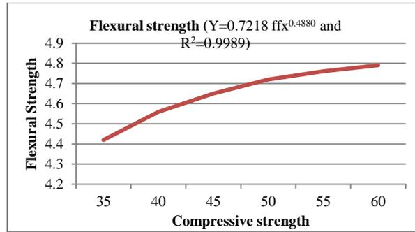
Fig 1.8 Relation between compressive strength and Flexural strength
