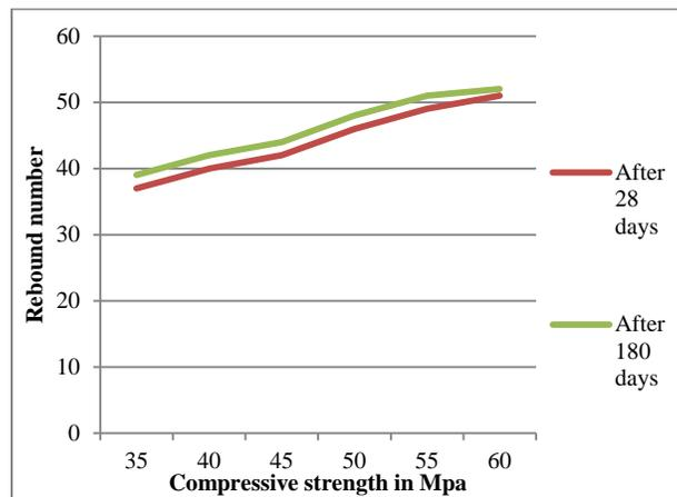
**Fig 1.1 Relation between rebound number and compressive strength**
