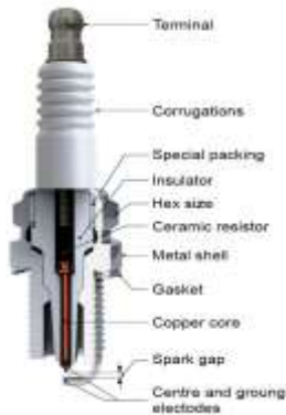
Figure (5): Spark Plug
